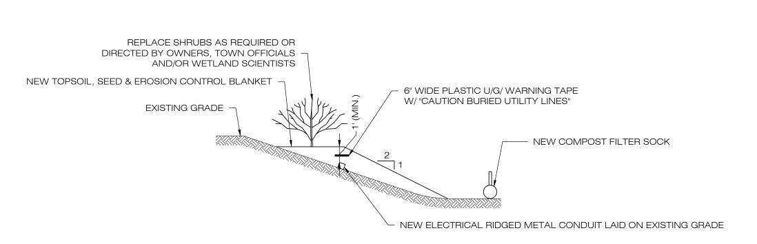
2 ELECTRICAL CONDUIT ON GRADE DETAIL
