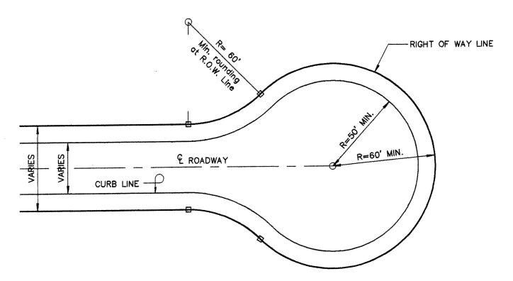
NOTE: THE CUL-DE-SACS SHOWN ARE ONLY TWO MINIMUM ARRANGEMENTS OUT OF MANY POSSIBILITIES. CUL-DE-SACS SHALL BE DESIGNED SO AS TO PROPERLY HANDLE THE TYPE AND AMOUNT OF TRAFFIC INVOLVED.
