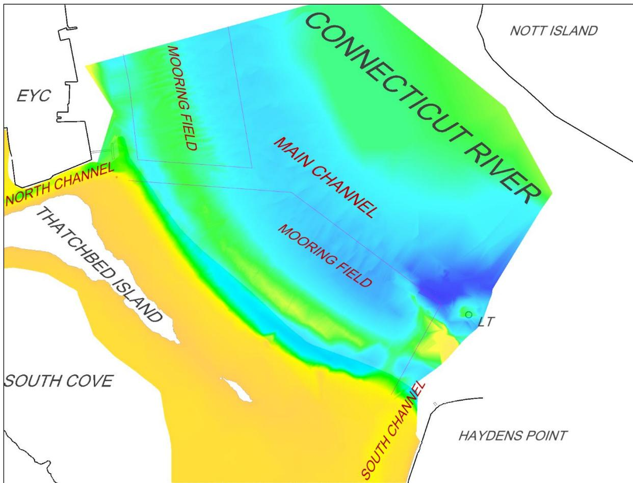
Figure 23: Main channel location, Connecticut River, north & south channels to South Cove. Color contours rendered from surveyed depths; see E-sized drawings for full detail.
