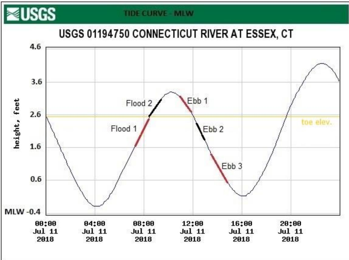
Figure 22: Survey line-cycle timing relative to tide curve for July 11, 2018. Note: Thatchbed Island toe of vegetation cut-bank approximate elevation 2.5 ft. MLW.
