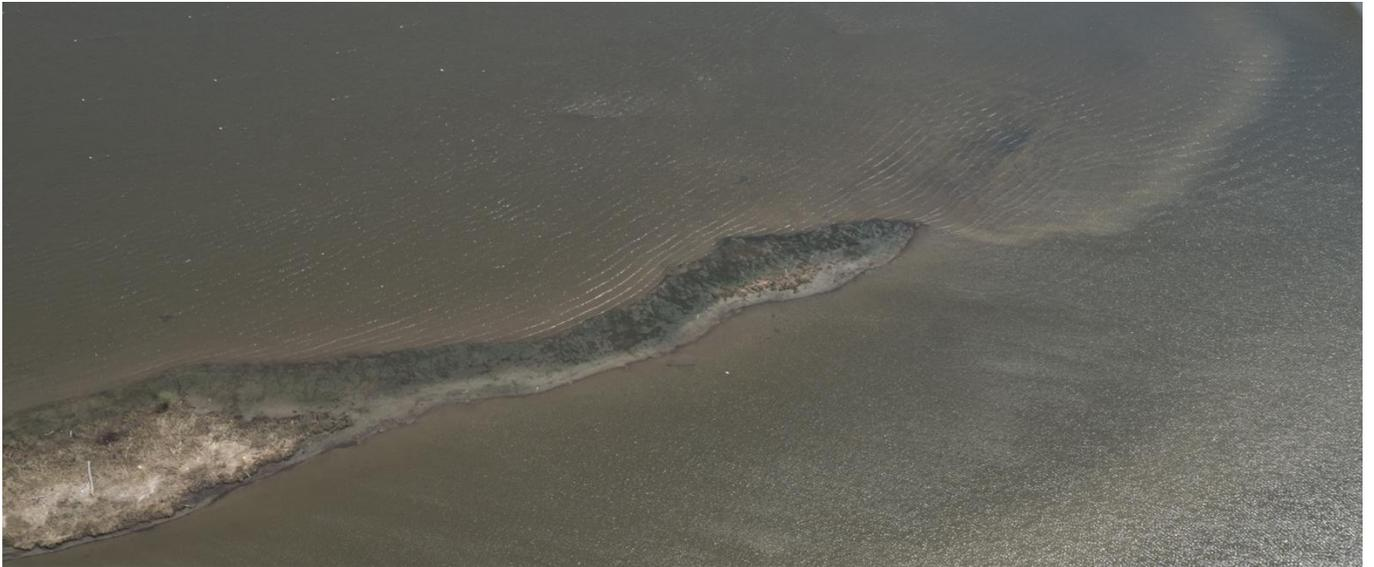
*Figure 4: Aerial view of boat wakes hitting easterly side of Thatchbed Island*
