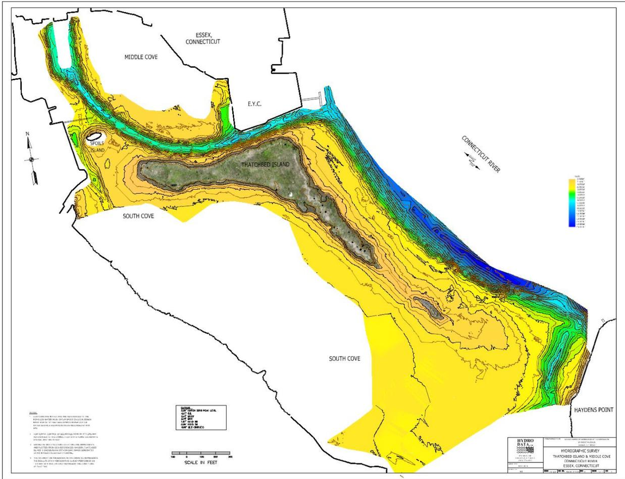
Figure 15: Thumbnail; Plan view hydrographic map of water surrounding Thatchbed Island, Essex, CT. For higher resolution, see full-sized drawings attached separately.
